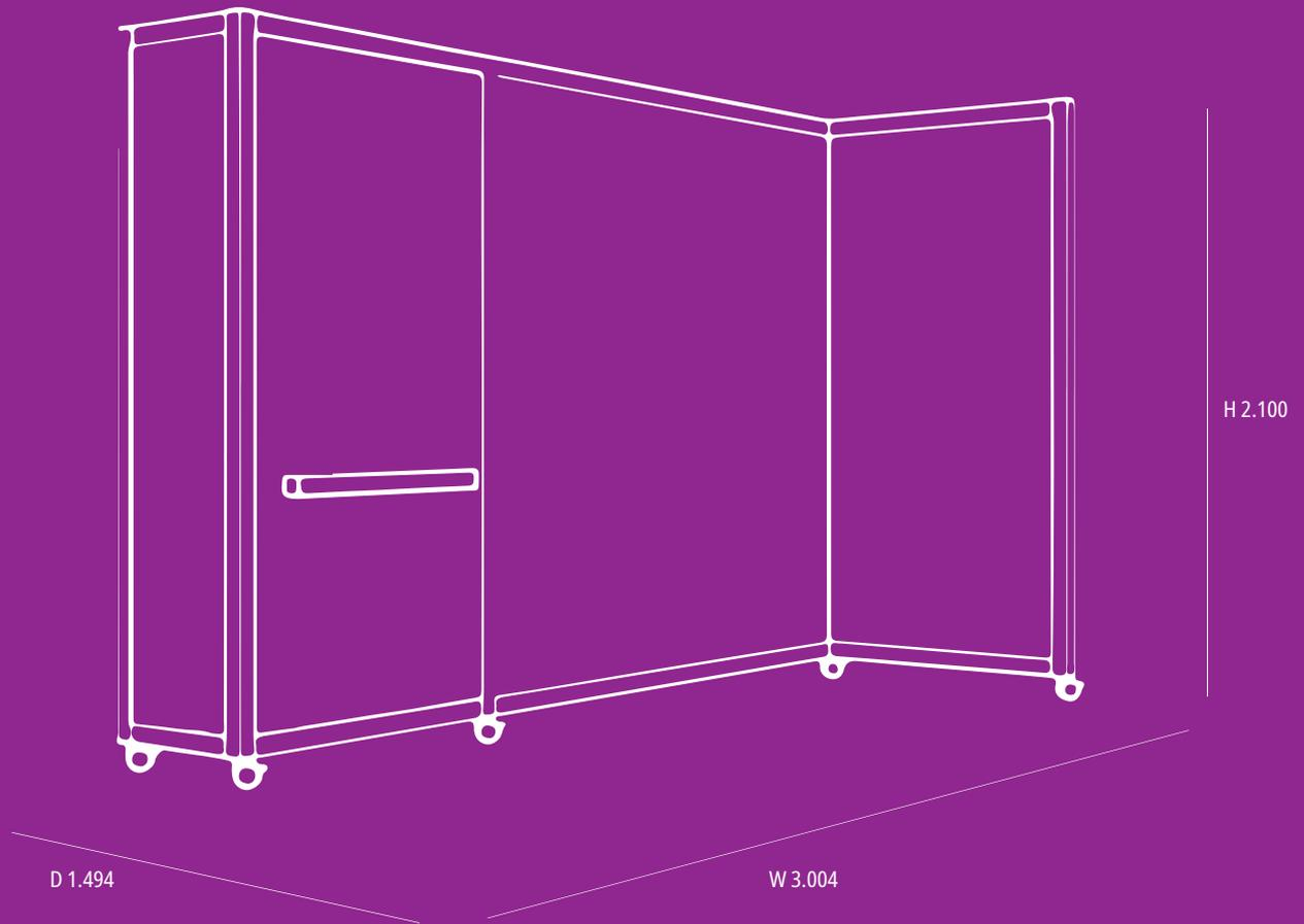
TECHEN: HxWxD 2.100x3.004x1.494mm, powder-coated aluminium, stainless steel, ECO-HPL, plastic.
