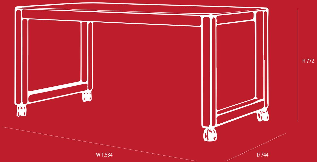
TIPPTOP: HxWxD 772x1.534x744mm, aluminium powder-coated, stainless steel, ECO-HPL, plastic.
