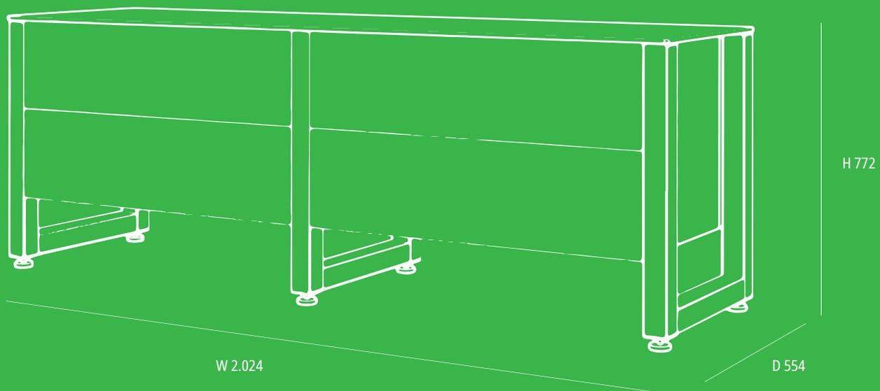
ANBORD: HxWxD 772x2.024x554mm, powder-coated aluminium, stainless steel, ECO-HPL, plastic.
